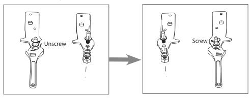
10.Refit the bracket fitting the bottom hinge pin. Replace both adjustable feet.
