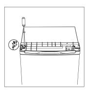
12. Put the top cover and fix it with 2 screws on the back.
