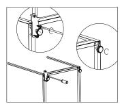
11. Place the door back on. Ensure the door is aligned horizontally and vertically, so that the seals are closed on all sides before finally tightening the top hinge.
