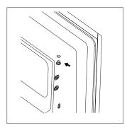
7. Rotate freezer door and place hinge side at left side. And then fix the door by holder.
