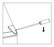
2. Undo the screws. Then remove the hinge bracket.
