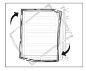
8. Refit the bracket fitting the bottom hinge pin. Replace both adjustable feet.
