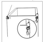
6. Unscrew and remove the bottom hinge pin, turn the bracket over and replace it.
