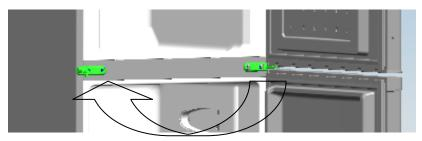
8、Set the bottom door right position, fix the mid-hinge.
