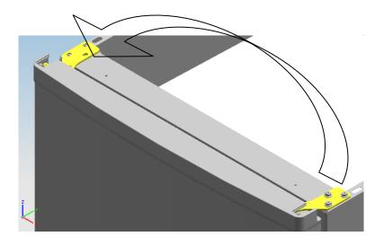
10、 Set the top door right position, fix the top-hinge and the cover.
