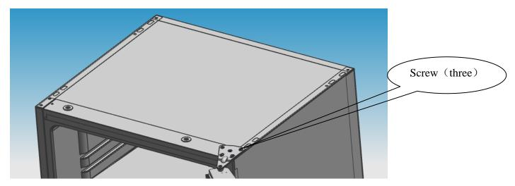
3 Replace the top-hinge and the top-door limit block and the door bearing bush to the other side.
