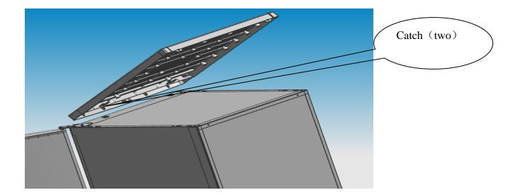
$2 \ _{\ }$  Remove the screws fixed the top-hinge with cross-ended screwdriver.
