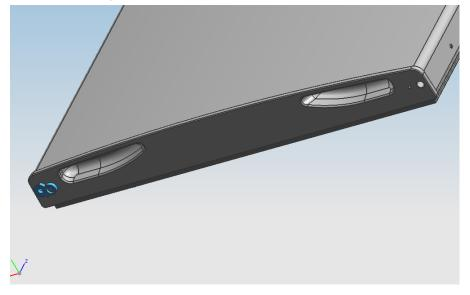
4. Disassemble the screws fixed the bottom-hinge with cross-ended screwdriver
