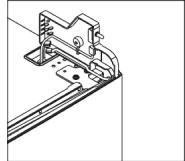
1 .Unscrew and remove the top hinge, and then remove the door.
