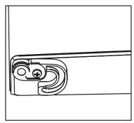
3 .Unscrew the bottom hinge, and remove the adjustable foot from the left side to the right side.
