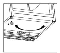
4 .Unscrew and move the bottom hinge pin from the right side to the left side, then install the bottom hinge on the left side of the appliance.
