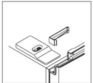
2 Unscrew right top hinge cover, and disconnect connectors of door switch and display.
