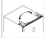
11. Install the top hinge to the left side, please slightly adjust the top hinge while installing to make sure gasket is well sealed.
