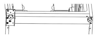
.Unscrew and move the top hinge pin from bottom side to upper side.Remove door switch from right hinge cover and then install it in left hinge cover which is placed in accessory bag.
