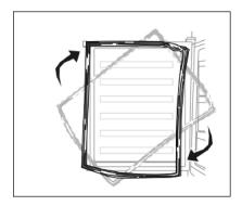
${\mathfrak n}$  .Install the door, and then move the connecting wires from right side to left side.
