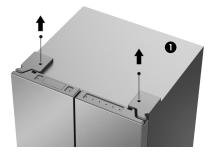
2. Remove the screws (2) fixed on the hinges with a wrench (5/16",8mm) and 1 ground screw (3) attached to the hinge with Philips (+) screwdriver. Remove the upper left and right door hinges (4).
