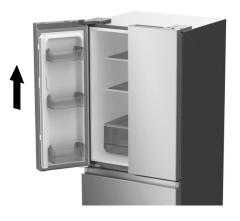
4. Remove the 4 hex head bolts hinges (5) with an Allen wrench (5/32",4mm). Remove the lower left and right door hinges (6).
