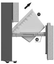
4. Remove the shelf(12) by pull it out between the beam and the slide guides.
