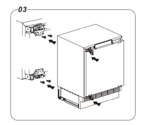
4. Replace the upper hinge cover (left and right). Replace the lower screw hole cover for the cabinet. Replace the screw hole cover for the door.
