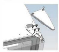
b) Unscrew the 4 screws that hold the upper hinge and remove it.
