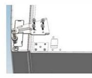
c) Loosen 1 screws as shown in the figure below, in order to remove the gap caver on the top side of the appliance.
