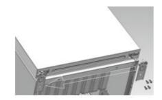
b) Install the shorter adjustable stand in the front on the side, where the lower hinge is. By turning the stand, you can adjust the height on this side of the appliance until it is levelled out.
