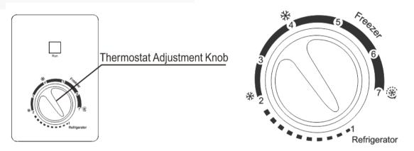
The inside temperature of freezer is regulated by thermostat adjustment knob.
