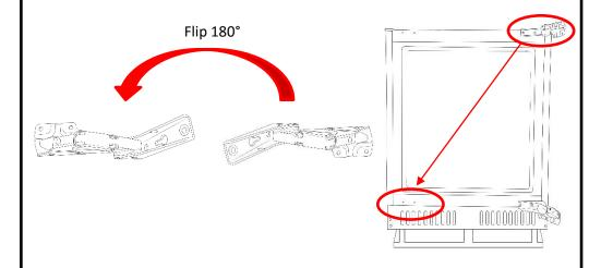
7. Repeat the previous step with the bottom hinge and then replace the screw hole covers on the opposite side.
