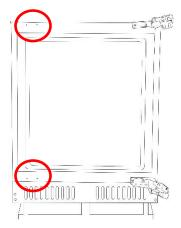
5. With the top hinge open, remove the screws from the top hinge that fix the hinge to the cabinet of the appliance.
