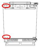
2. With the door closed remove the screws from the top and bottom hinges that hold the appliance door to the hinges. Remove the screws from the top hinge first.
