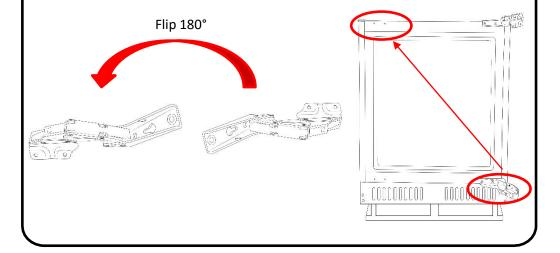
8. Reattach the door by fixing the outside screws of the hinge to the door. You must ensure the fridge door is aligned horizontally and vertically, so that the seals are closed on all sides before finally tightening.
