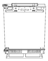
9. Replace the 4 screw hole covers on the cabinet of the appliance at the top and the bottom on the opposite side of where the hinges are now fixed.
