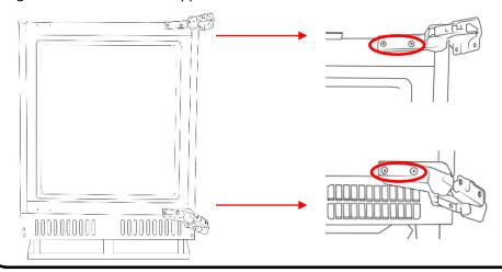
6. Flip over the top hinge (by 180°) and fix it in place on the diagonally opposite corner of the appliance cabinet.
