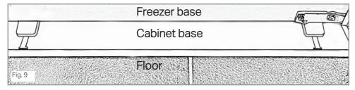
With the base of the appliance aligned correctly with the edge of the cabinet base, the metal trim at the top of the appliance should sit flush against the cabinet edge (if it does not, ensure the base is aligned as per Fig. 9 and that the metal trim in Fig. 10 is not damaged).
