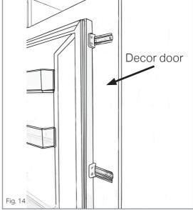
Important: After completing the installation, check that the appliance is secured within the unit and that the door(s) close and open properly. If there is no resistance from the door seals when opening the doors, then it is probable that the appliance and/or decor doors are not fitted properly.
