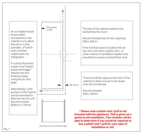
The open channel at the rear is clearly shown. For the correct operation of the appliance it is important that the top of the housing unit is not blocked off. A channel depth of 40-50mm is normal with most units.
